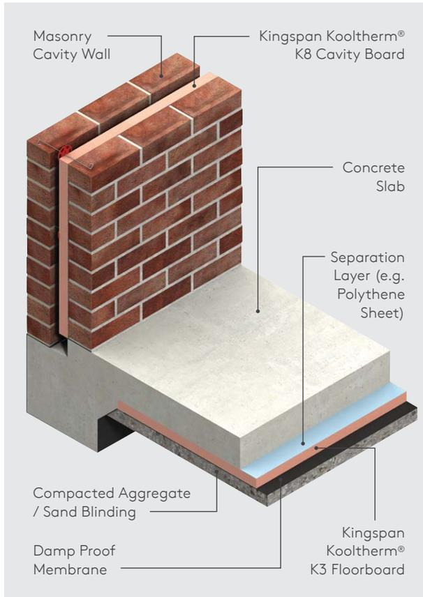
Figure 1. Solid residential concrete slab on ground floor with Kooltherm® K3 Floorboard below the floor slab.
