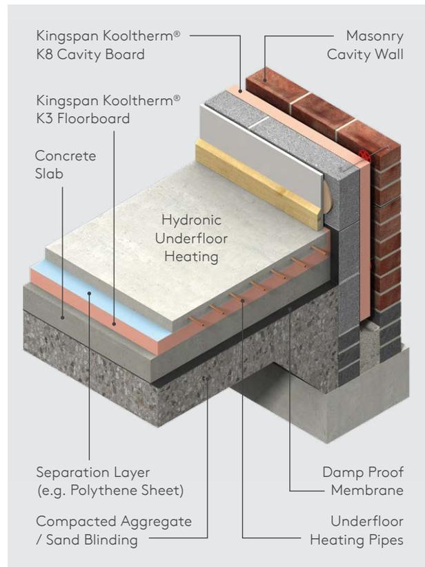
Figure 2. Residential concrete slab with hydronic underfloor heating on ground floor with Kooltherm® K3 Floorboard over the floor slab.
