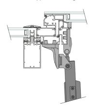
Roof windows, outward opening, side installation
