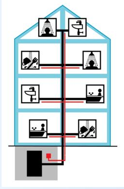
Self-regulating cables are simply taped to the supply piping and insulated. The cable can be cut to length and terminated on site without the need for special tools.
