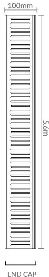
\* Total length is 5.8m, total usable length is 5.6m to allow for any wastage during the anodising process.
