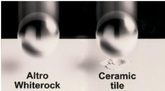
The impact 'drop' tests were conducted using a 322g steel ball (tested to BS EN 438 standard) released from various heights (min. 25 mm) on to both a ceramic and Altro Whiterock surface (flat face, joint, edge and corner).
