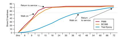
The above graph shows how the Shore D develops many times more quickly than traditional epoxies, which gives the Mastertop® Fast Return to Service its unique attributes. Along with strength and hardness gains, it also attains its full chemical resistance in the same time period.
