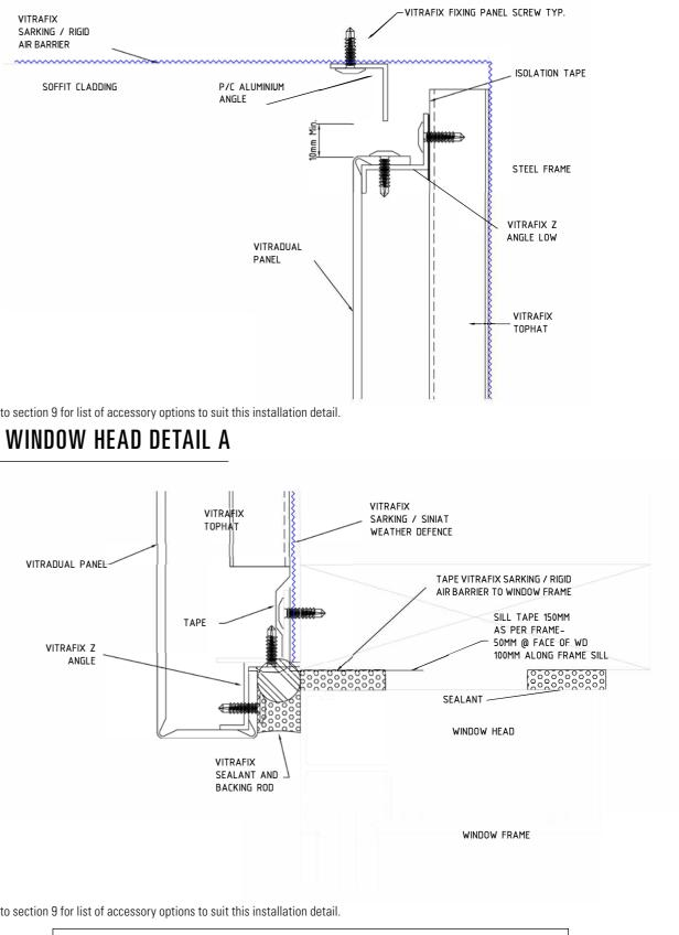
DISCLAIMER: These details are limited to the generalized design specification for Vitradual, and are intended for use by a technically skilled person only. Use of the same is at their own discretion and risk.
