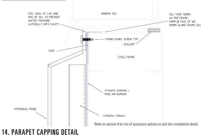
CORNER BRACED WITH CLEAT (TYP) RETURN SARKING OVER THE TOP OF THE PARAPET CONTINUOUS SILL FLASHING FOR RIGID AIR BARRIER VITRAFIX SARKING / RIGID AIR BARRIER VITRAFIX FIXING PANEL SCREW VITRADUAL PANEL VITRAFIX TOPHAT
