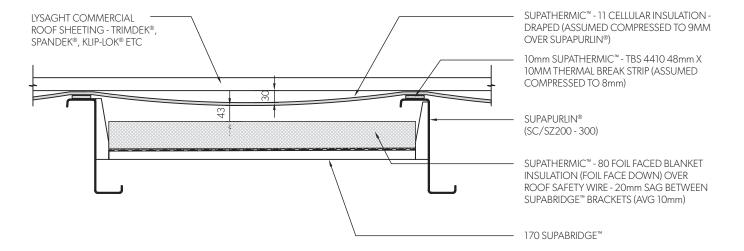
Values are calculated for each project based on the project combination of purlin size / spacing and roof pitch.
