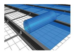
SUPATHERMIC<sup>™</sup> - MR Sarking maybe screw fixed to SUPABRIDGE<sup>™</sup> members during installation to aid placement.
