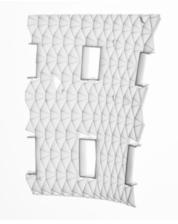
This complex facade is parametrically designed based on a sun path analysis, and would be incredibly difficult to fabricate by any other means at such a scale.
