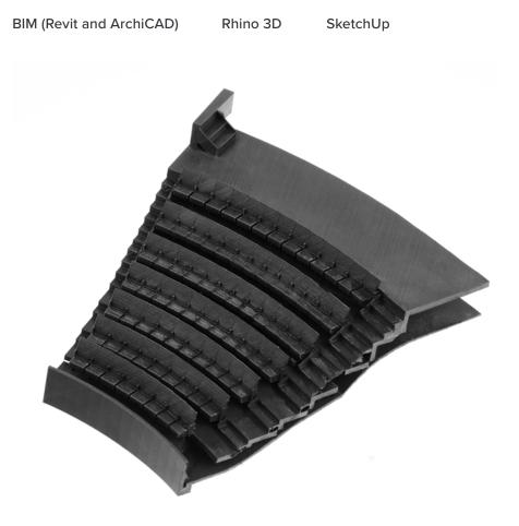
This auditorium section was 3D printed as one single piece on a Form 2 with Black Resin. **Model by DLR Group.**
