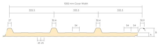
**Note:** Dimensions are nominal. Actual dimensions will vary due to manufacturing tolerances. Precise dimensions must always be measured from actual samples. All measurements in mm.
