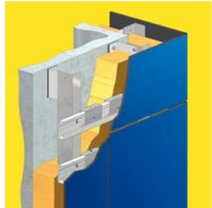
Invisible fixing with brackets on rails
