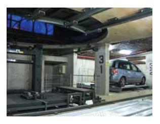
The pallets are made of galvanized sheet steel and are used to transport the car in the parking. Each pallet is assigned to a determinated parking place. The pallets are moved by independent drive groups that transfer them from one to another parking area.
