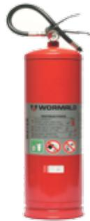
Foam fire extinguishers, marked with a blue band, work by covering a burning flammable liquid with a blanket of foam, cutting off the fire's air supply and preventing the release of flammable vapours.
