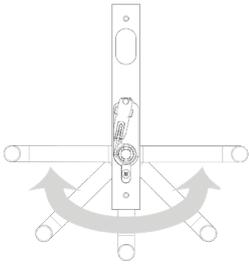
Handing of the lever is a simple operation: rotate the lever to the desired handing and then guide the spring mechanism into the channel.
