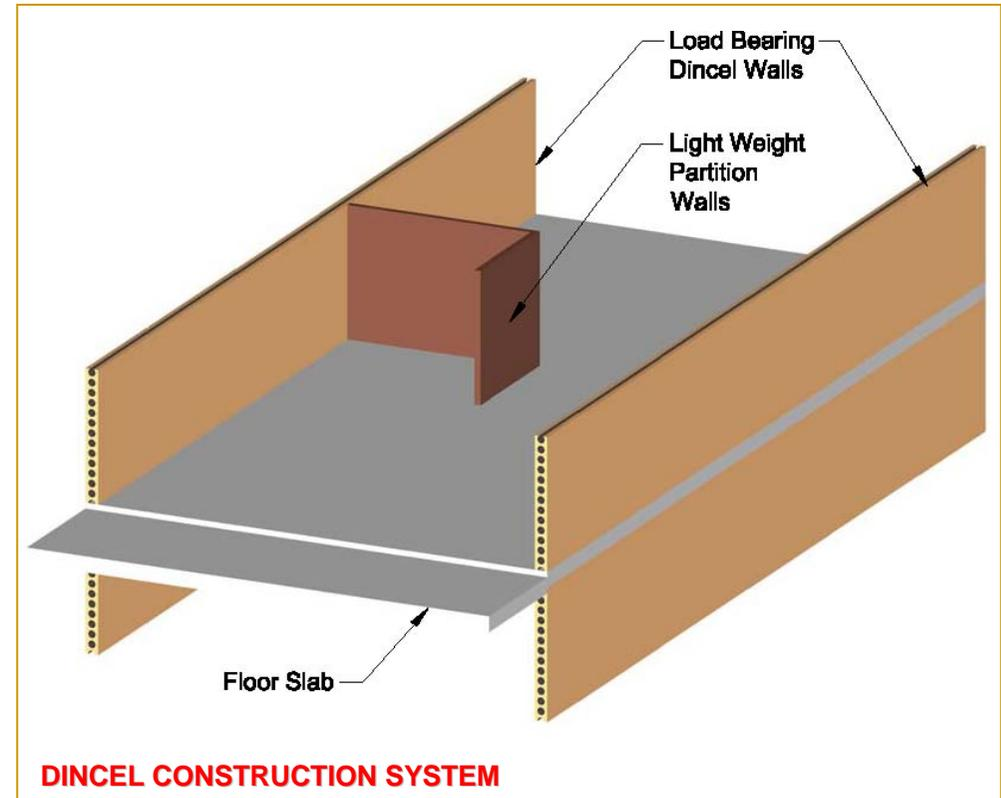
**FLOOR SLABS CARRIED BY LOAD BEARING DINCEL-WALLS
