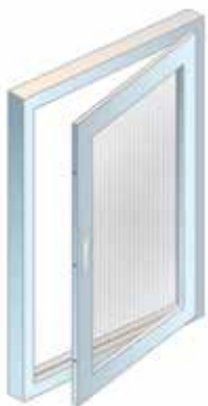
Hinged windows can open inward or outward.
