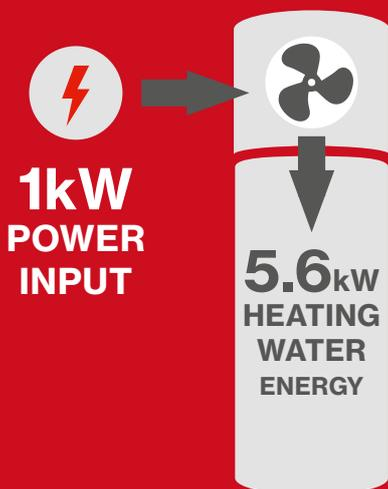
At 20°C ambient temperature, water heated from 15-55°C
