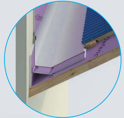
Box gutter details
