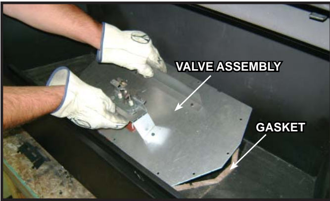
Figure 16.6 Remove Valve Plate
