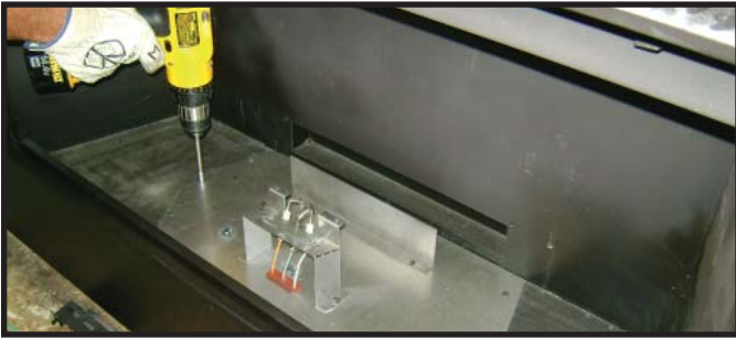
Figure 16.5 Remove Valve Plate Screws
