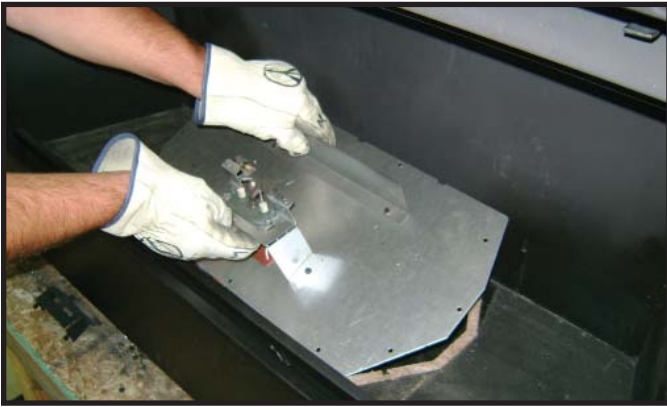
Figure 11.3. Remove Valve Plate
