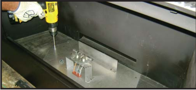
Figure 11.2. Remove Valve Plate Screws
