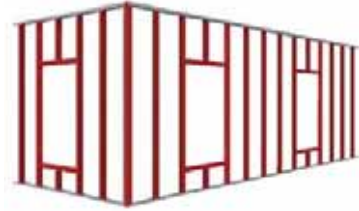
Construction of extreme walls
