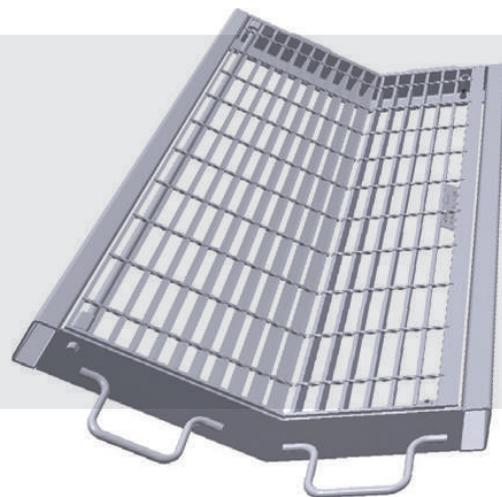
These grates are specifically designed to suit the roll of the kerb and are used predominantly in sub-divisions. All grates are hinged for easy access and bolted down to deter unwanted access. The frame comes with reo concrete tie-ins for easy tying into your formwork prior to casting. These grates meet the respective load class requirements of AS 3996:2019 as detailed in the table below.
