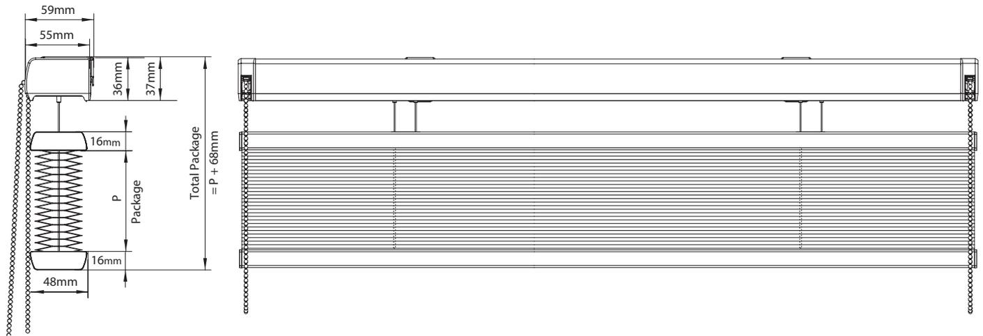
Universal Installation Bracket - Face or Reveal Fixing
