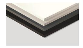
EGGER Compact Laminates coloured core are compact laminates according to DIN EN 438-9 with a coloured core based on curable resins. They have a multilayer structure and consist of melamine resin impregnated decorative paper and multiple layers of soda craft paper impregnated with phenolic resins, which are laminated under high pressure and heat.
