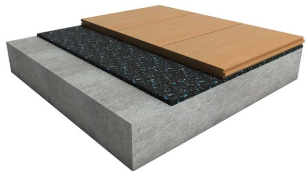
Typical bamboo floor system includes approved Regupol adhesives. Refer to bamboo flooring acoustic system for more technical information.
