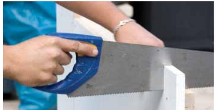
Hand sawing is suitable for general cutting operations and for small cuts, notchings or small penetrations. However, this method of cutting can be rather time intensive. The fastest way is to allow the saw to work at its own speed, trying to force the tool to cut faster merely blunts the teeth.
