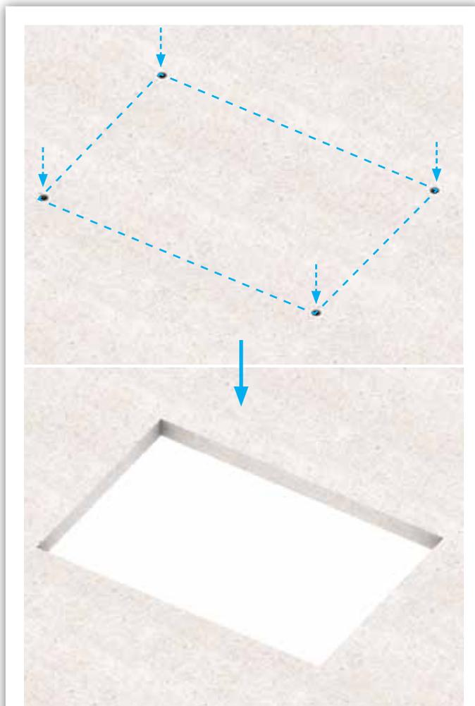
Apertures opening using alternative method: Never make holes by using heavy hammers, cold chisels or other "aggressive" methods. This will damage the underside of the boards and adversely effect the fi re performance of the system.
