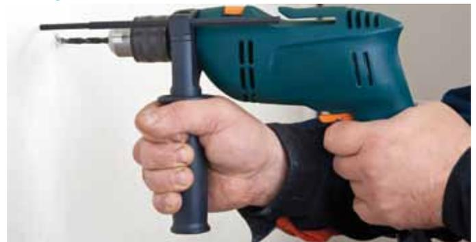
Drilling can be carried out either by hand drill or any conventional power drill with or without dust extraction. For best results, the boards should be firmly supported behind the location of the holes. Generally when working on PROMATECT® 100 boards, the use of drills with point angles of 60° to 80° rather than the more usual 120° type, are preferable and more efficient.
