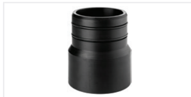
GEBERIT HDPE STRAIGHT ADAPTER (MALE) TO COPPER For connection of Type B copper pipe with inner diameter of 98mm to Ø110mm PE pipe. Available in size Ø110mm.
