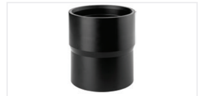
GEBERIT HDPE STRAIGHT ADAPTER (FEMALE) TO COPPER For connection of copper pipe with outer diameter of 101.6mm to Ø110mm PE pipe. Available in size Ø110mm.
