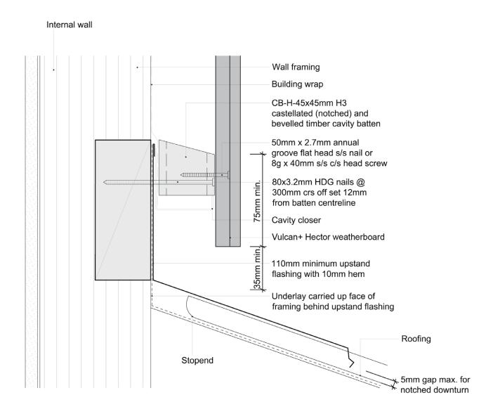
Note: refer to NZBC E2/AS1 Table 7 for apron flashing cover over roofing
