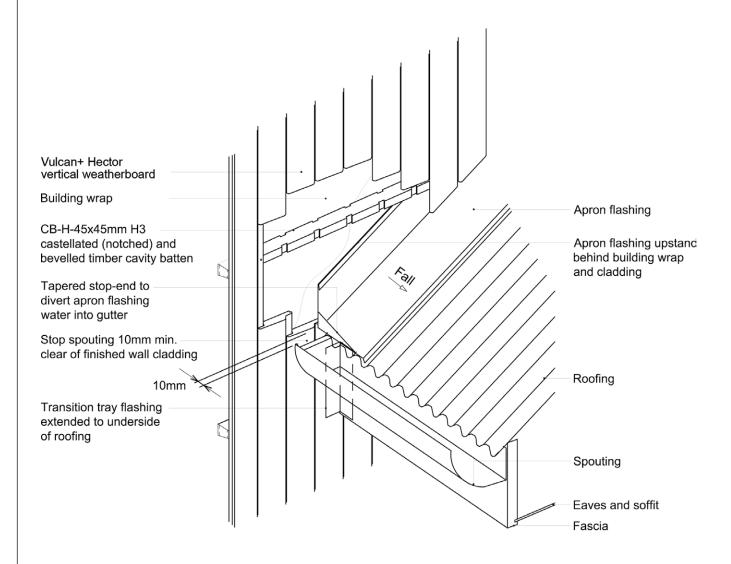
Note: refer to NZBC E2/AS1 Table 7 for a pron flashing cover over roofing  $\,$
