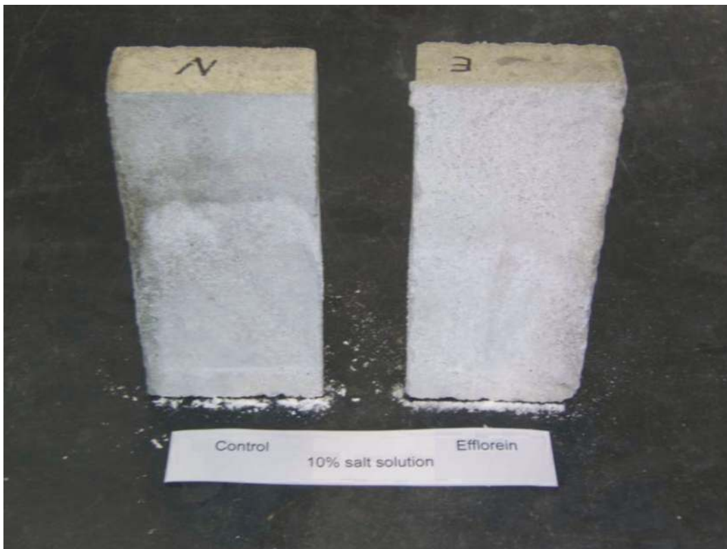
Photo 4: Specimens after 3 days in 10% salt solution, then air-drying
