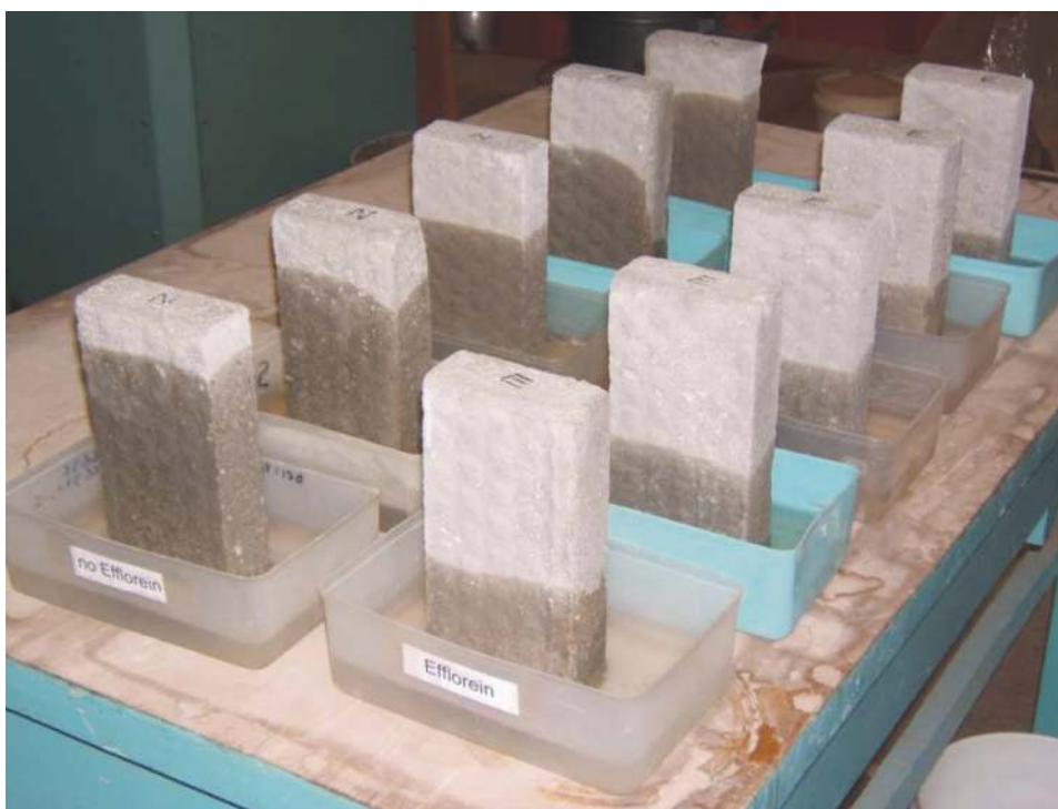
Photo 1: Control and Efflorein specimens after 18 hr in 1% salt solution
