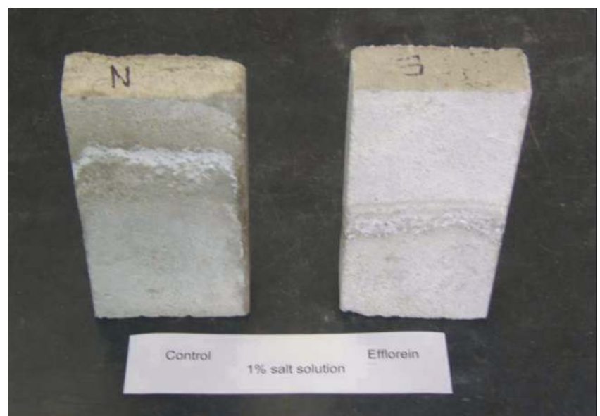
Photo 2: Specimens after 4 days in 1% salt solution, then air-drying
