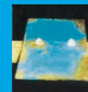
Chlorinated rubber coating: Rust at the corners
