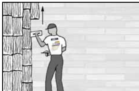
(diagram.2) transfer texture to the wall
