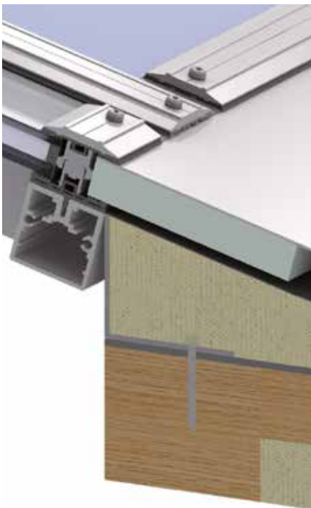
INSTALLED ON A TIMBER UPSTAND
