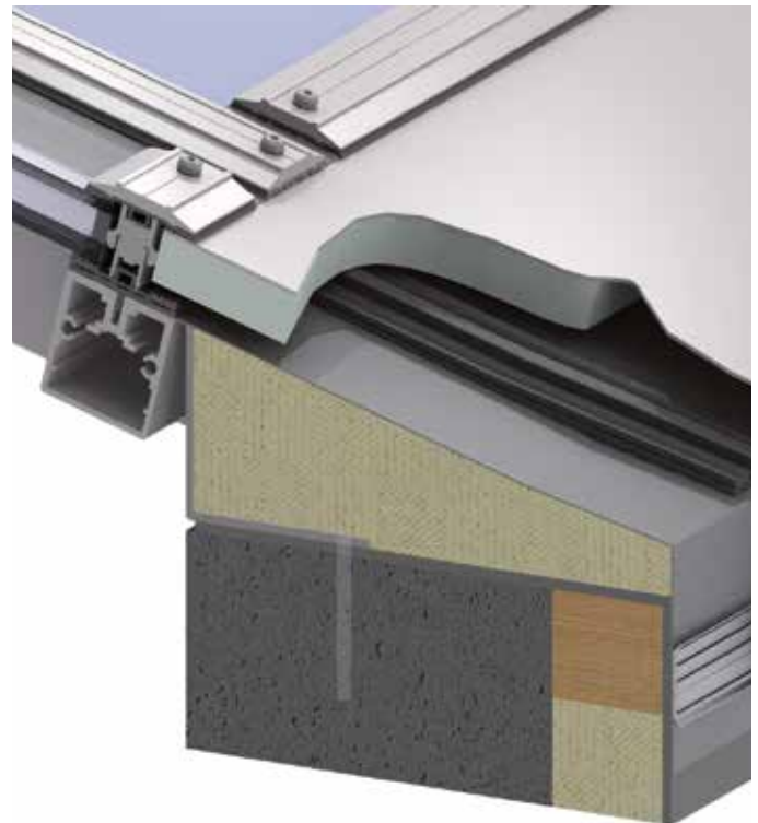
INSTALLED ON A CONCRETE UPSTAND
