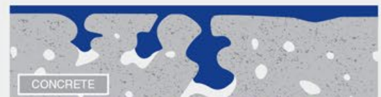
MICROSCOPIC CLOSE UP OF CONCRETE SURFACE USING A FILM FORMING SEALER
