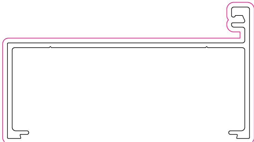
WAWF011 FLAT JAMB Anodised Perimeter = 433 Paint Perimeter = 230 I_{xx} = 9.770 \times 10^4 \text{mm}^4 I_{yy} = 7.479 \times 10^5 \text{mm}^4
