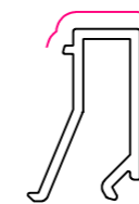
WAWF008 SINGLE GLAZED BEAD Anodised Perimeter = 106 Paint Perimeter = 100 I_{xx} = 8.739 \times 10^2 \text{mm}^4 I_{yy} = 2.732 \times 10^3 \text{mm}^4
