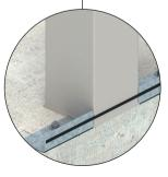
A VJ2 EPDM bubble gasket is required at each vertical panel joint detail to provide an air seal. Apply gasket to the vertical steel member. At corner locations VJ2 EPDM bubble gasket to be equally positioned on each flange. VJ2 EPDM bubble gasket to lap over drip flashing by min. 20mm
