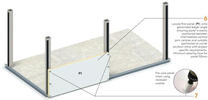
Install 3 No. primary fastener with recessed washer, approximately 50mm down from horizontal panel joint to each panel end (minimum).
