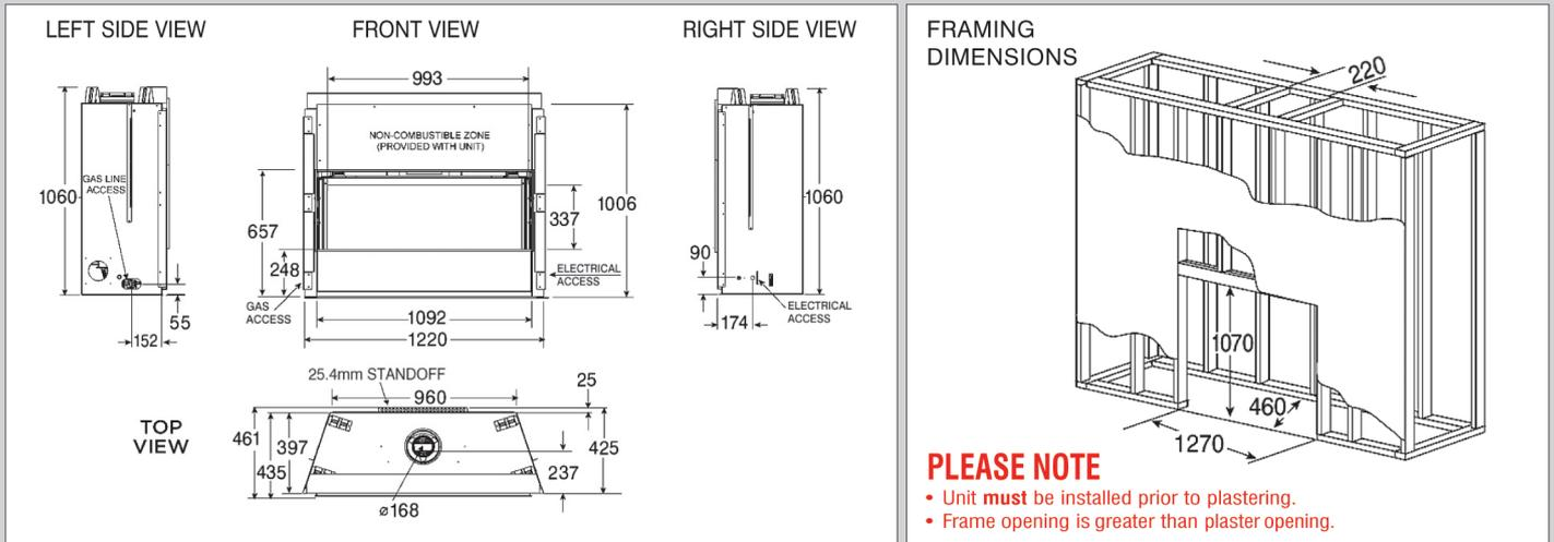
Dimensions shown above are in millimetres. Reference dimensions only. We recommend measuring individual units at installation. Assume the use of 10mm plaster.
