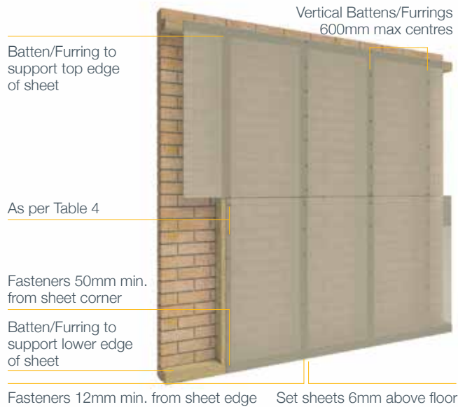
FIGURE 5 – INSTALLATION USING BATTENS/FURRINGS
