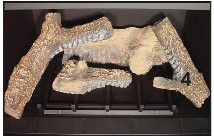
→ LOG #4 (SRV385-722): Place log #4 on 5th grate tines and rest its top into the groove on log #1.
