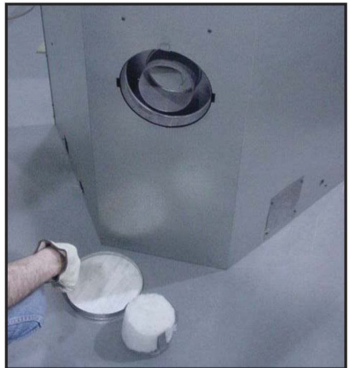
Figure 9.10 Discard the vent cap, remove and discard the insulation basket.
