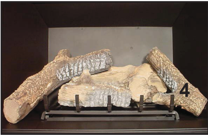
→ LOG #4 (SRV385-722): Place log #4 on 5th grate tines and rest its top into the groove on log #1.
