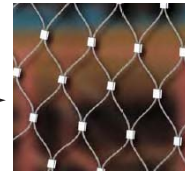
Webnet with 60deg mesh angle.
