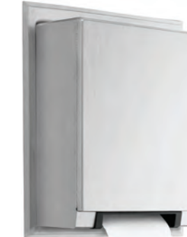
B-29744 Semi-Recessed Automatic Roll Paper Towel Dispenser Satin Finish Stainless Steel 435 W x 515 H x 130 D Dispenses 205 W x 244 M Rolls Electronic Sensor & Controls
