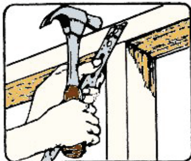
Hammer fixing to top plate
