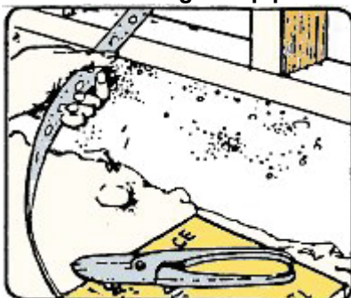
Pulling Out The Brace
