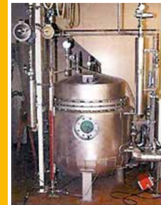
Schematic of the pressure vessel with test specimens vertically arranged in oxygen-enriched water.
