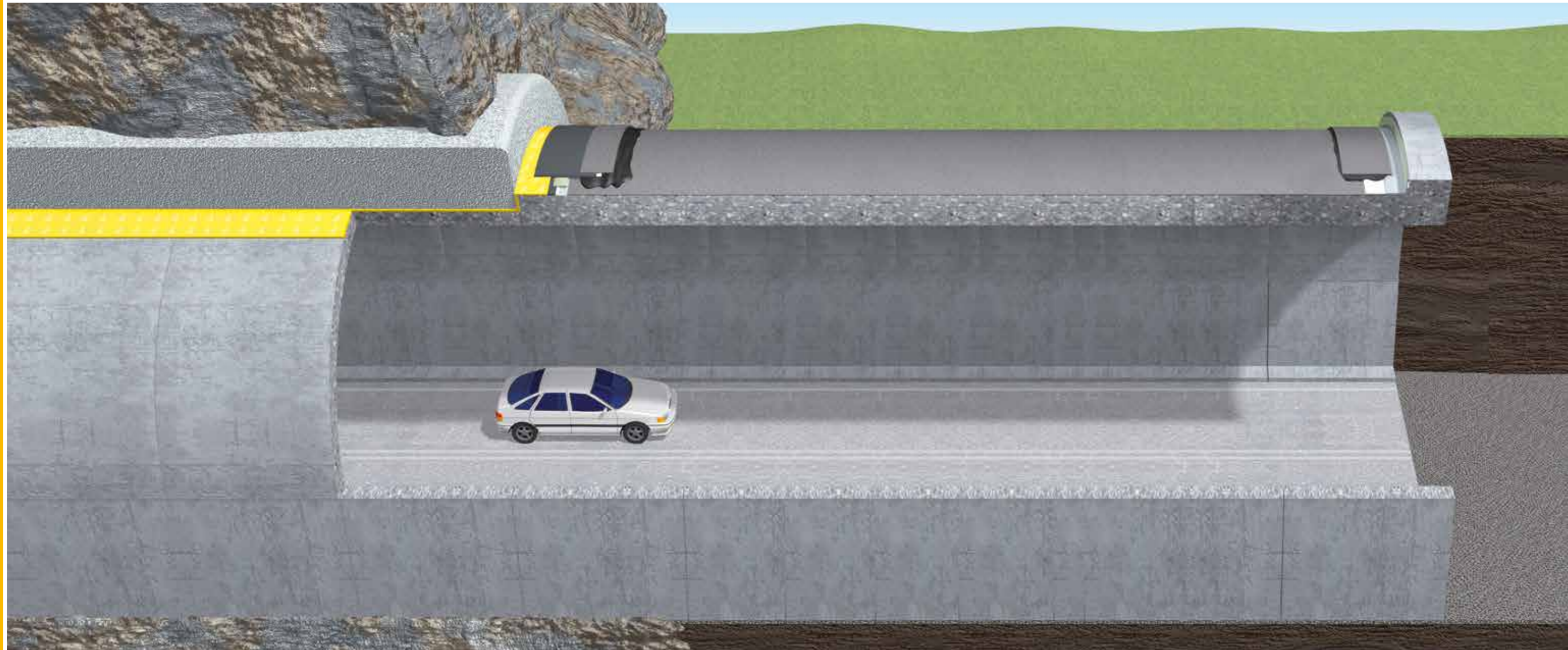
Drainage of Mountain Water / Not holding a Head of Water / Drill-and-blast / TBM Excavation
