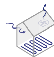
System E+®: Natural supply, demand- controlled mechanical extraction with heat recovery for domestic hot water and heating.
