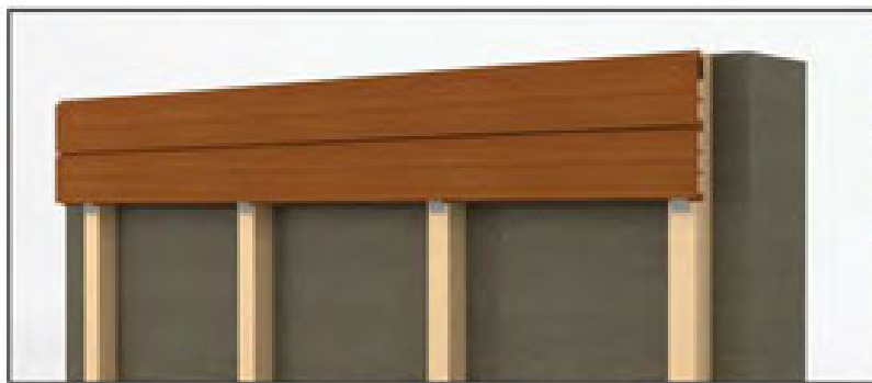
QBI-09 and QBI-16 Second Board Installation
