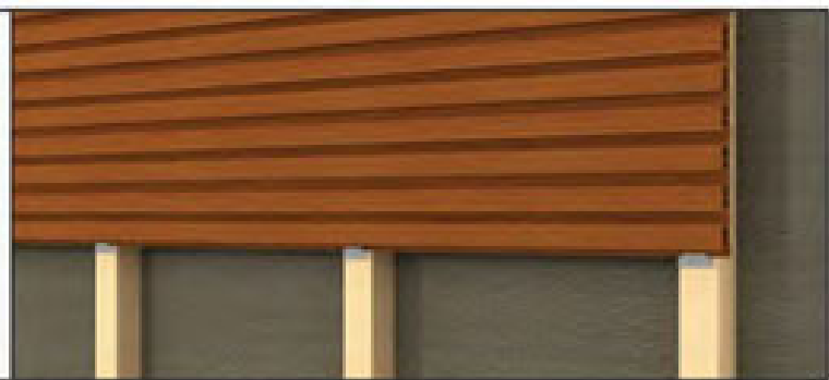
THO-26 Second Board Installation
