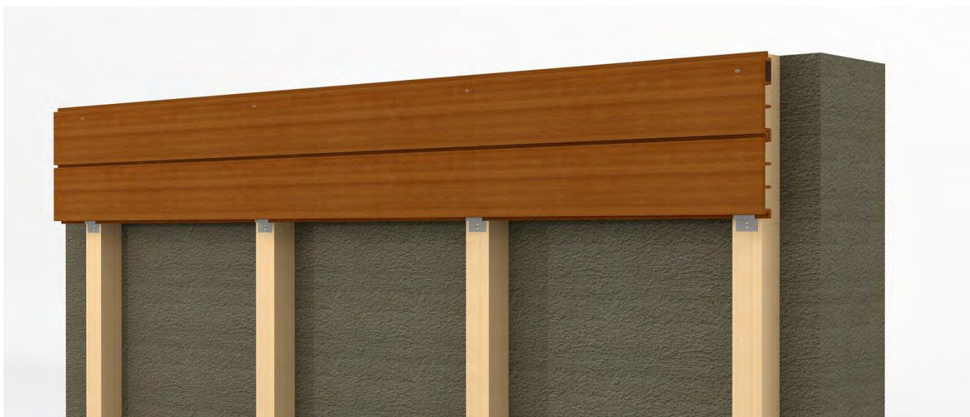
Figure 5 - QBI-09 and QBO-16 Second Board Installation
