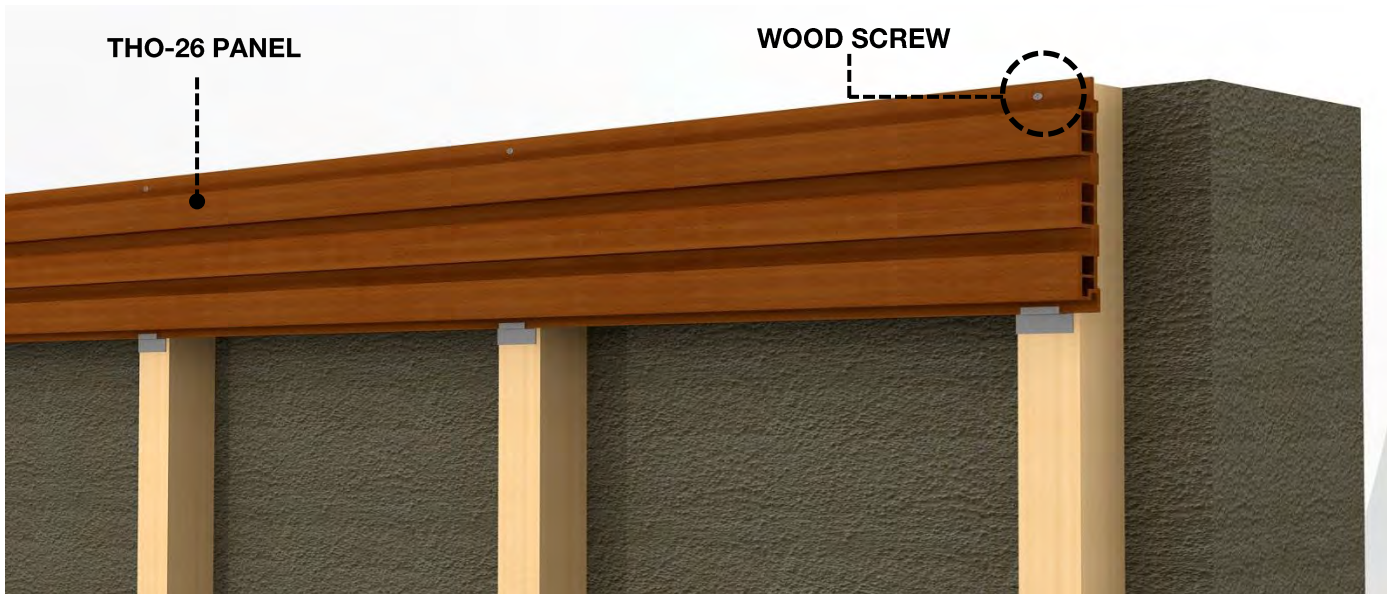
Figure 7 - THO-26 First Board Installation
