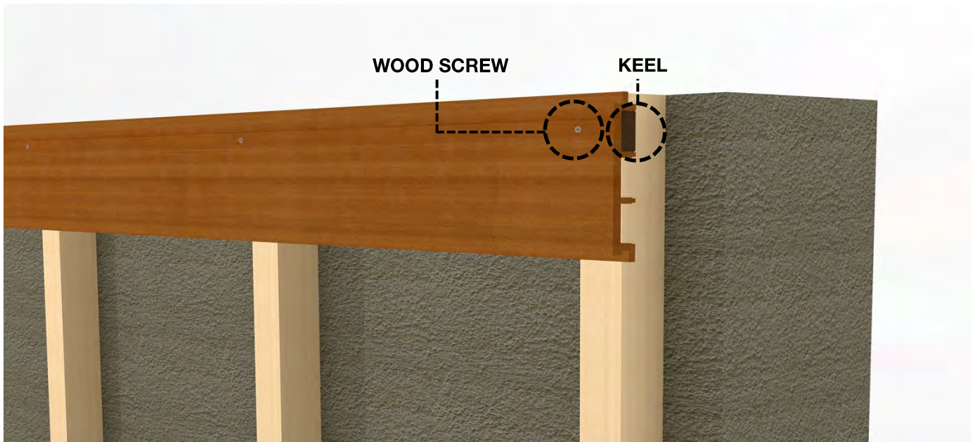
Figure 3 - QBI-09 and QBO-16 First Board Installation
