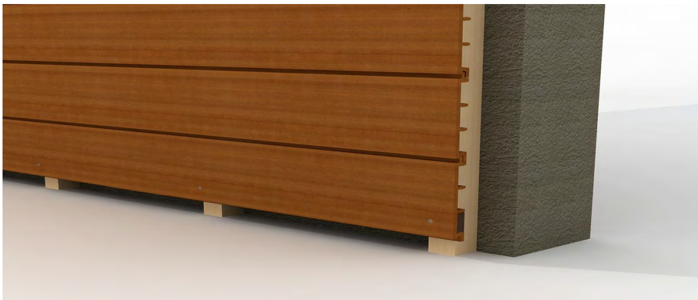
Figure 6 - QBI-09 and QBO-16 Last Board Installation
