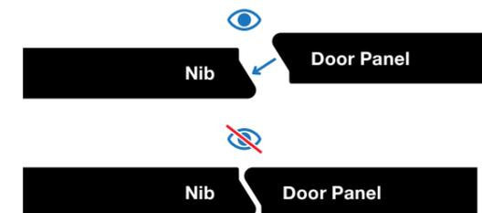
No edge strip required as compact laminate black core is visible on the edges
