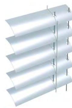
with wire tensioning, opened by 45°
