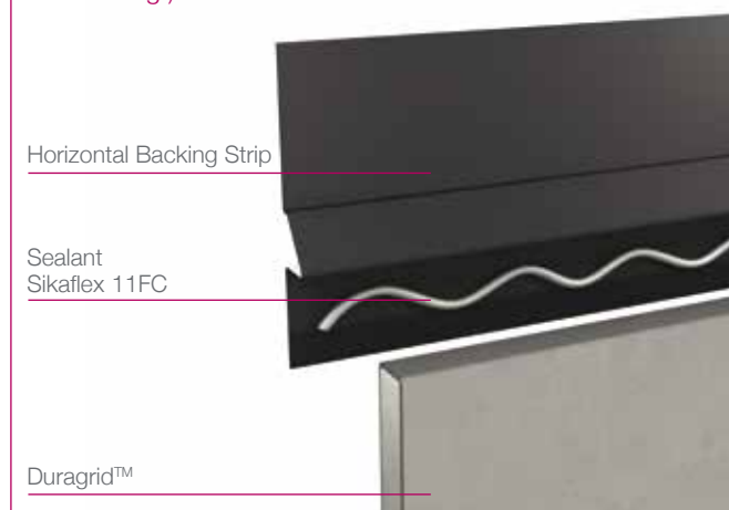
Figure 3 Sealant (Preferred Option for Optimal Adhesion and Sealing) - Front View
