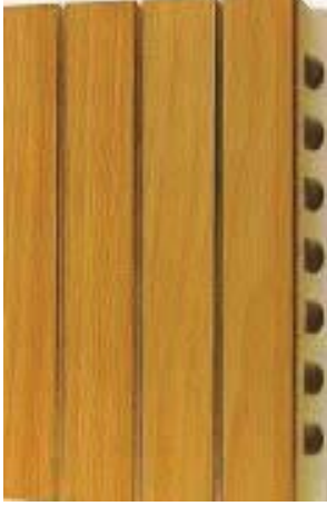
3mm Grooves at 32mm Centres. Code G32 NRC 0.68 (0.76) (0.71)
