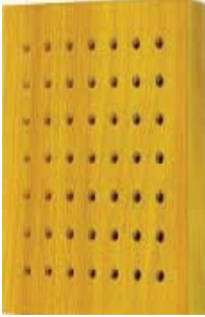
6mm Holes at 16mm Centres. Code P616 NRC 0.72 (0.88) (0.85)
