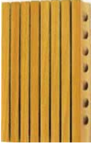
3mm Grooves at 8mm Centres. Code G8 NRC 0.77 (0.96)
