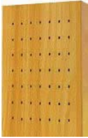
3mm Holes at 16mm Centres. Code P316 NRC 0.59 (0.70)
