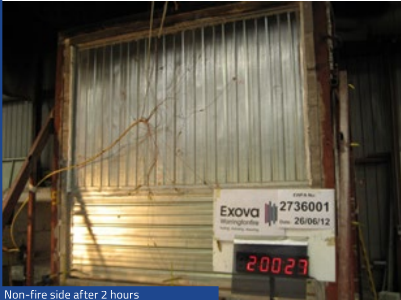
Non-fire side after 2 hours
