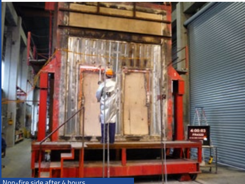
Non-fire side after 4 hours
