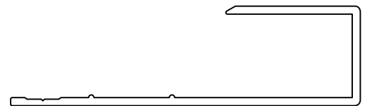
UA4532 - Window Flashing
